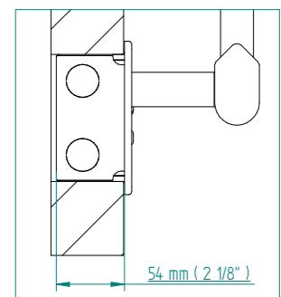
Ingombro placchetta a muro / Wall-plate dimensions /
